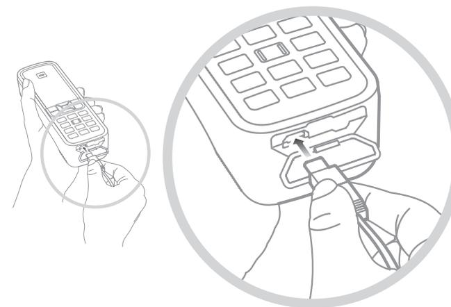
Connect the charger to a power source and the micro USB connector to the port at the base of the phone, under the USB/audio protective cover.
