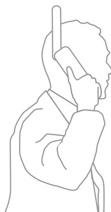
Stand outside with a clear view of the sky with the phone antenna pointing upwards. There must be a clear line of sight between the phone's antenna and the satellite.
